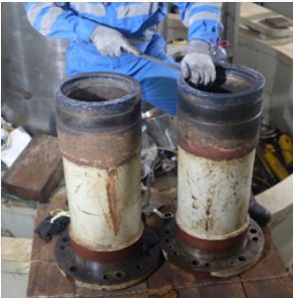
Figure 11: Inspection of the upper mantle plate under the 54G1 Head Cover
